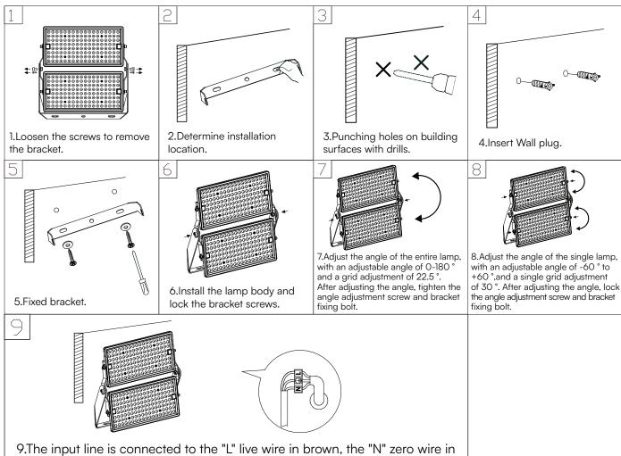
9.The input line is connected to the "L" live wire in brown, the "N" zero wire in blue, and the yellow green wire is connected to the ground wire. After connecting the wires, it is necessary to use insulation tape and waterproof tape for insulation and waterproofing treatment. It is recommended to use a professional waterproof junction box
