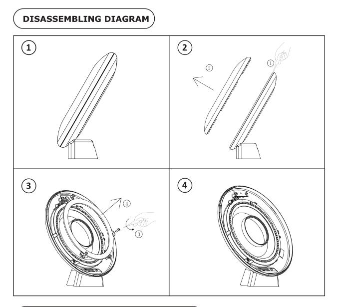
HOW TO DISASSEMBLE THE DEVICE
